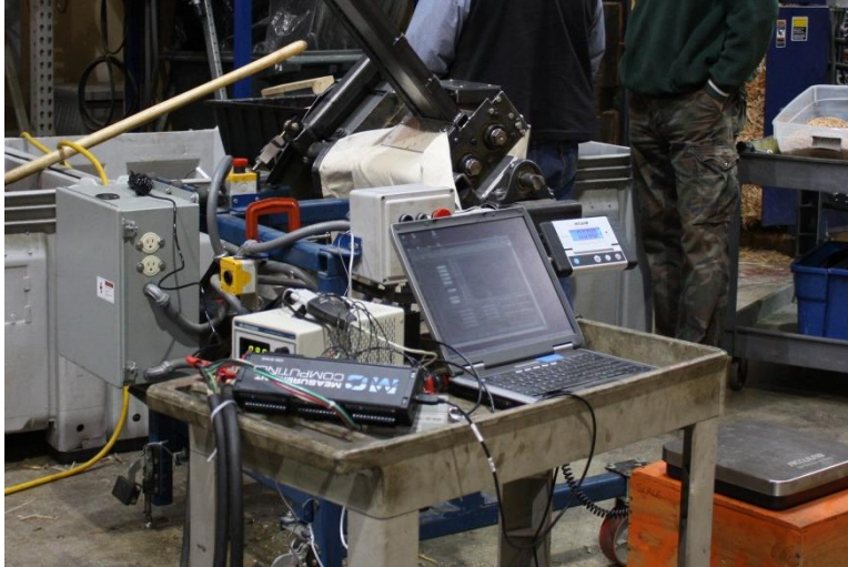
Figure 5. Data logging system: Measurement Computing USB-1616HS DAQ board, Laptop running LabView with custom vi, power supply, and electrical power scaling box (scales line voltage to acceptable DAQ input voltage).
