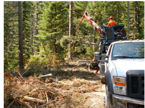
Figure 4. Forest Concepts' engineering prototype forest utility baler collecting forest residuals from roadside windrows on Snoqualmie National Forest.
