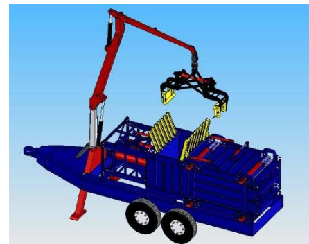
Figure 1. Concept rendering of forest utility baler on straight trailer and with 17-ft reach self-loader.
