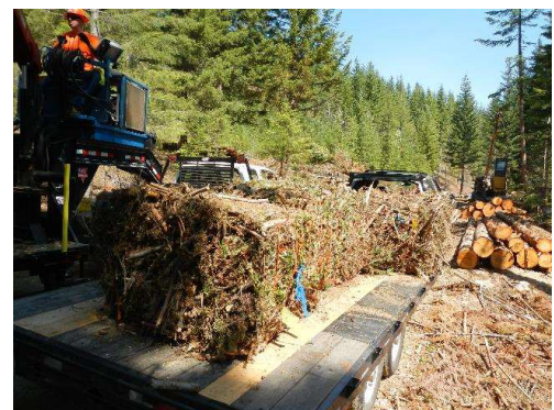
Figure 5. Forest residuals bales produced by utility baler from roadside windrows on Snoqualmie National Forest.
