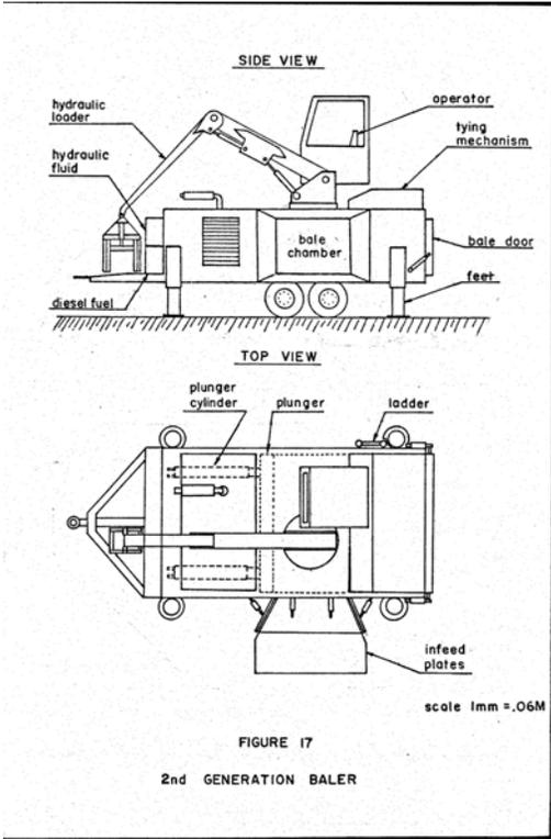
**Figure 3.** Concept sketch for VPI second generation baler. (P. Schiess)
