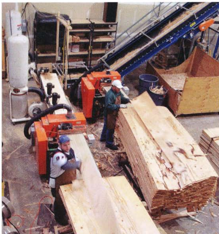
Employees of Forest Concepts hand-feed wood veneer into the muncher for conversion into WoodStraw.
