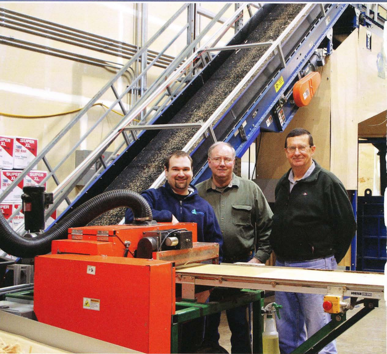
Dave Lanning, Jim Dooley and Mike Perry, left to right, stand next to the "muncher," a machine that makes Forest Concepts LLC's patented WoodStraw erosion control material.
