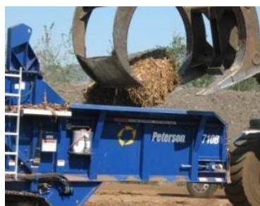
Figures 5. (Left) Moving bales in grinding yard. (Center) Grinding with horizontal grinder. (Right) Ground bale to produce boiler fuel for use by Avista Power in Kettle Falls Generating Plant.
