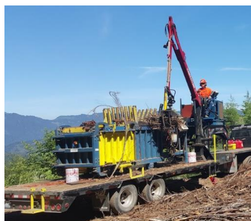
Figures 1. (Left) Conceptual rendering of chipper-replacement woody biomass baler for use by arborists and vegetation management contractors. (Right) Forest Concepts' engineering research prototype baler mounted on 5 th -wheel grapple trailer.
