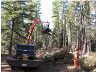
Figures 3. Forest Concepts' engineering prototype baler collecting roadside thinnings in central Oregon from a wildfire protection shaded fuel break project.
