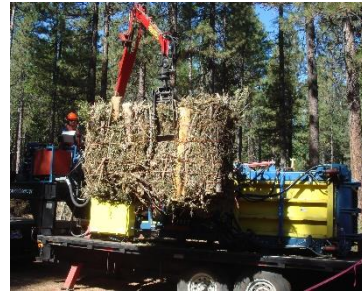
Figures 3. Forest Concepts' engineering prototype baler collecting roadside thinnings in central Oregon from a wildfire protection shaded fuel break project.
