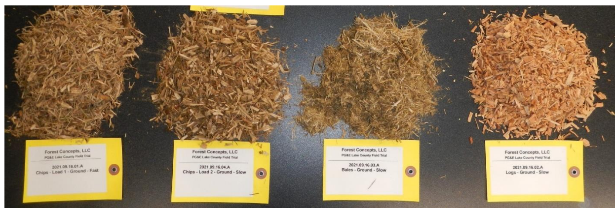
Figure 2: Feedstocks after grinding and screening to pass a 3/8-inch round hole screen and be retained on a 3/32-inch wire screen using Forest Concepts’ orbital screen system.
