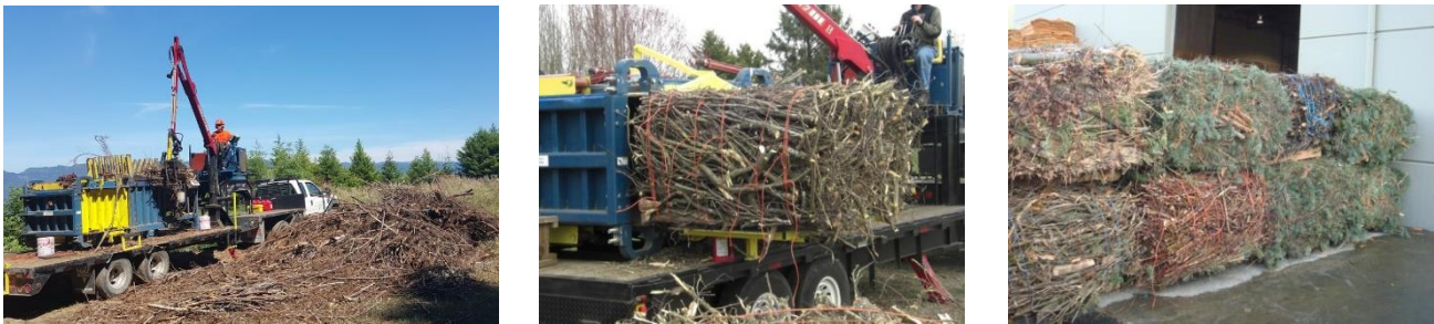
Figure 1. a) Forest Concepts prototype forest residuals baler; b) completed bale; and c) stack of baled woody biomass
