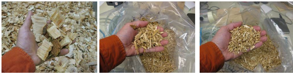
Figures 5a, 5b, and 5c. Whole tree chips as received, results of one pass through 4.8mm wide rotary shear, results of two passes through 4.8mm wide rotary shear.
