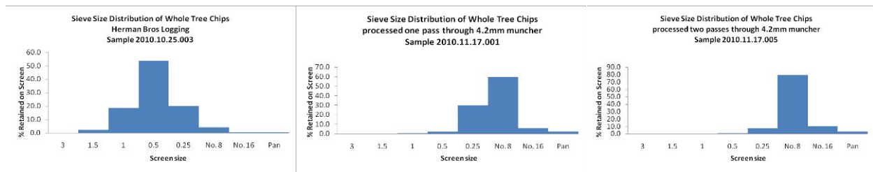
Figure 7. Histogram of particle sieve size distribution for raw chips, single pass and two pass through the rotary shear muncher. (Percent retained is on a mass basis)
