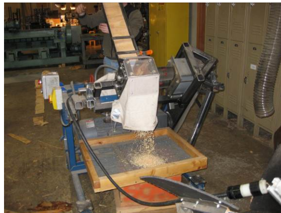
Figures 4. Forest Concepts' laboratory rotary shear machine (muncher). Shown here processing veneer strips.
