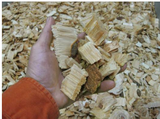
Figure 1. Handful of chips with bin of whole tree chips in the background.
