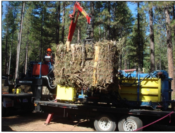
Figure 1. Baling of forest residues on the Deschutes National Forest (Forest Concepts photo).
