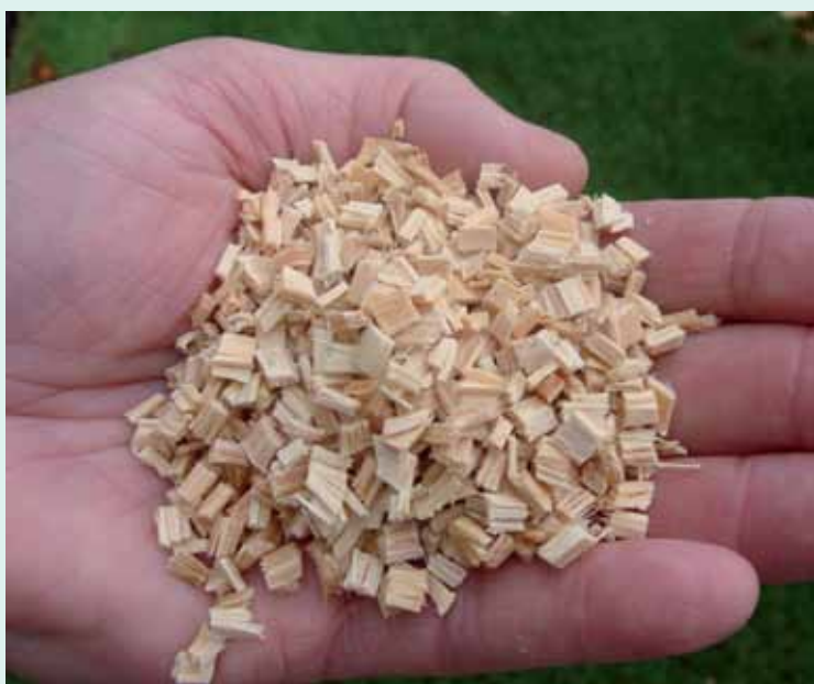
Figure 2. Wood feedstock particles 4.8-mm long made from 4.2-mm fir veneer using a prototype Crumbler™ machine.
