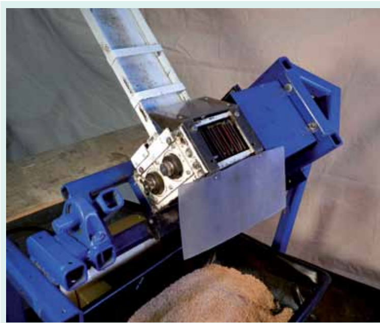
Figure 1. Forest Concepts laboratory Crumbler™ showing the infeed chute and feedstock particles in collection tray. Reproduced with permission from Forest Concepts © Forest Concepts, LLC.
