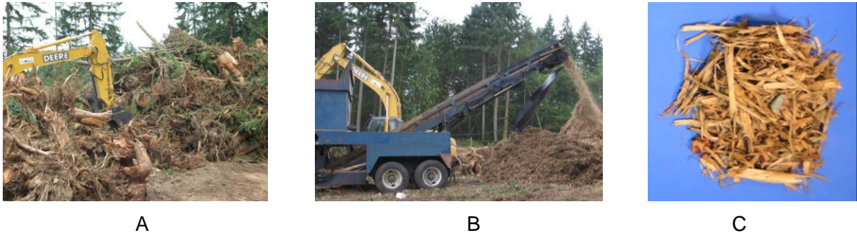
Figure 1. Land clearing debris woody biomass (A), grinding biomass (B), and clean woody biomass feedstock from ground land clearing debris (C).
