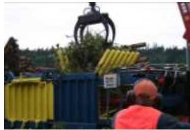
Figures 3. Field trial of prototype biomass baler at BRC Inc. yard waste facility in Auburn, WA.
