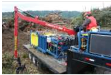
Figures 3. Field trial of prototype biomass baler at BRC Inc. yard waste facility in Auburn, WA.
