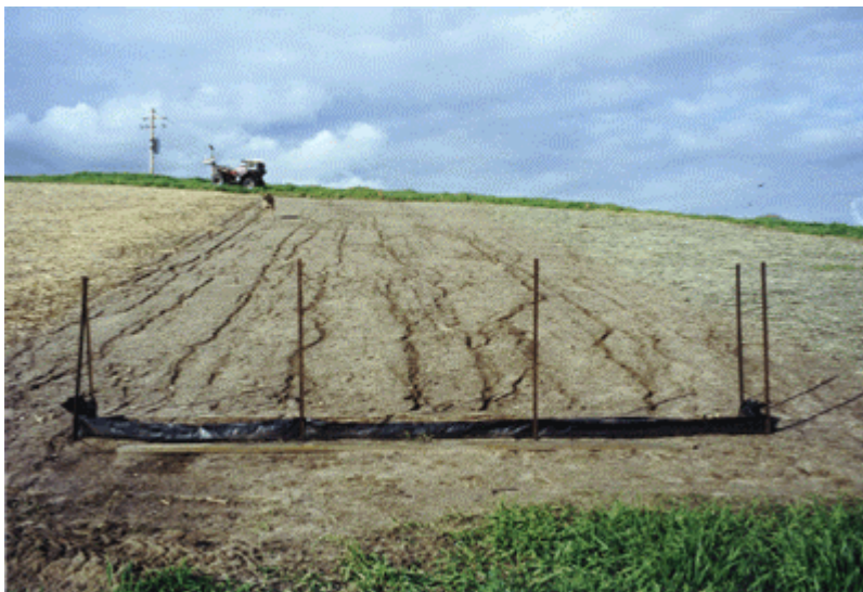
Figure 10: Ernst site on January 3, 2005 with wood-strand plot on the left, bare soil in the center, and barley straw plot on the right. As of this date, neither of the treated plots showed any signs of rill erosion.
