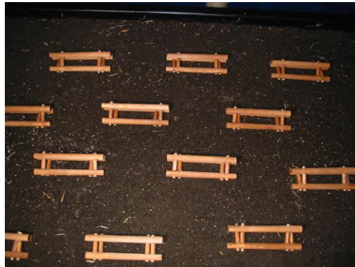
Figure 9. FlowCheck™ model structures deployed as single units in a regular pattern across the slope. Note that ends slightly overlap to reduce the risk of rill formation.
