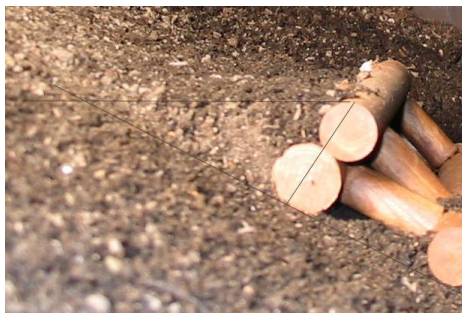
Figure 3. Concept model of hillslope erosion control structure is shown on 60 percent slope. The volume of sediment stored is approximately equal to the area of the triangle minus the cross sectional area of one pole.
