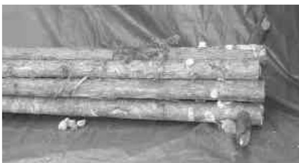
**Figure 1 a,b,c,d.** A small model was used to prove the concept of building large diameter structures from pairs of small diameter logs. A full-scale prototype was fabricated from forest residuals using a mix of western red cedar, hemlock, alder and Douglas fir logs.
