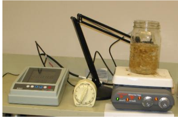
Figure 1 Simple experimental set up with EC meter, timer, and hot plate stirring device.
