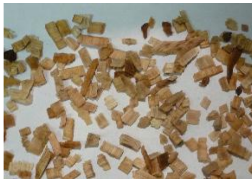
Figure 6. Sample of conifer microchips produced by commercial scale drum chipper.
