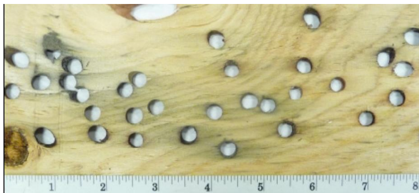
Figure 8. Wood veneer containing saltwater worm holes.
