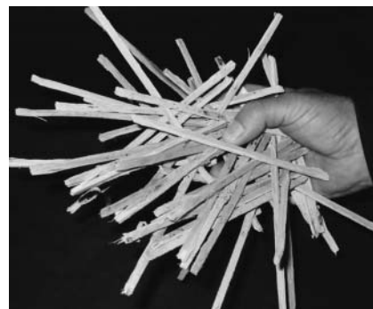
Wood-strand width, length, thickness, and blend are designed to provide functional performance. WoodStraw™ mulch includes a blend of sliced veneer strands based on lab and field research results.
